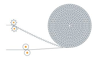
As well height (gap between wraps) increases, the amount of heat transfer and pressure drop is reduced. The decrease in well height increases the transfer of heat and pressure drop. In EVO-R Compact Air Handling Units, condensing type rotors with a 1.6 mm well height are used as standard. For higher heat transfer requirements, rotors with 1,4 mm well height can be selected from the selection software ,well heights of 1,8mm, 2,0mm and 2,5mm are available for lower pressure drop requirements.
